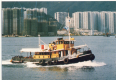
High-horsepower use of Isotta fuel in tug which operates between Hong Kong and mainland China. The vessel is powered by a 160-hp Isotta engine, 4470hp at 1,000 rpm.
