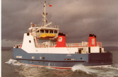
One of a fleet of boats operating in the south of Scotland powered by twin Kubota D602 engines. Each engine developing 120 hp at 1,800 rpm.
