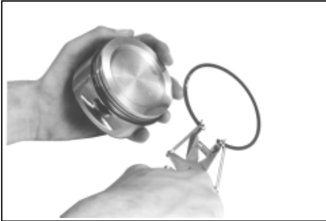
Figure 10-10. Installing Piston Rings With Expander.
