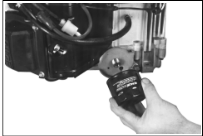
Figure 9-4. Removing Oil Filter.
