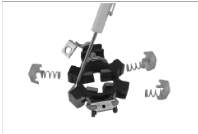
Figure 8-36. Removing Retaining Clips.
