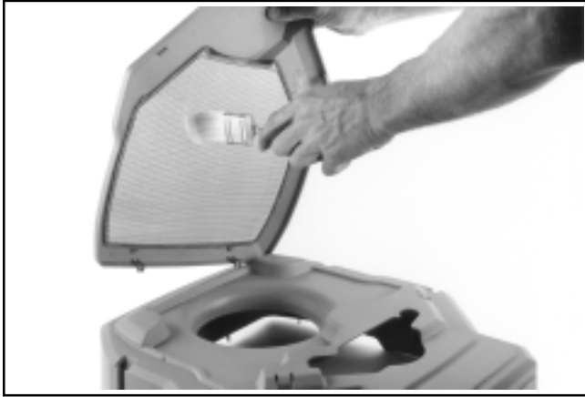
Figure 4-4. Cleaning Separated Screen Assembly.
