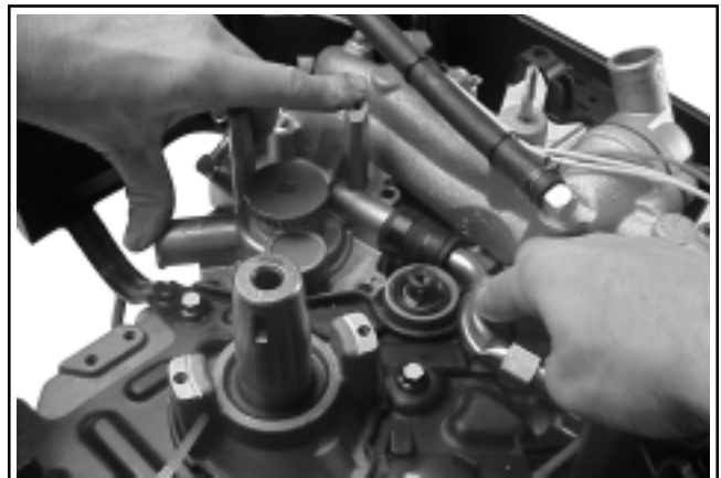
Figure 11-64. Pushing Down on Pump and the Tube for Installation.
