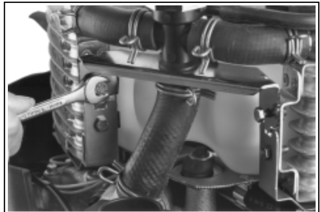
Figure 7-6. Loosening Retainer Bracket Mounting Screws.
