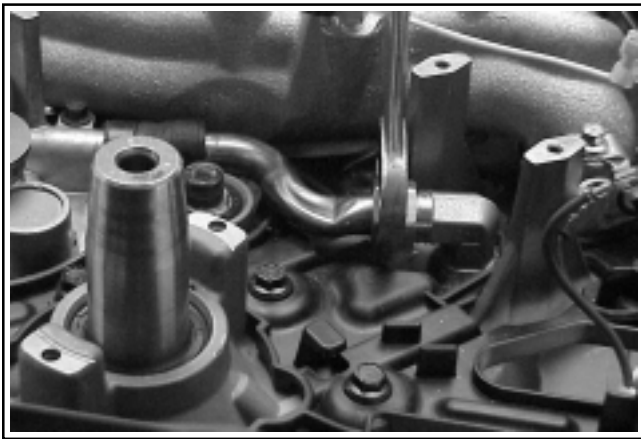
Figure 9-44. Removing Hex. Cap Section.
