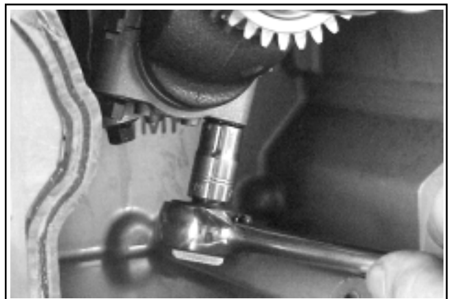
Figure 9-77. Removing Connecting Rod End Cap.
