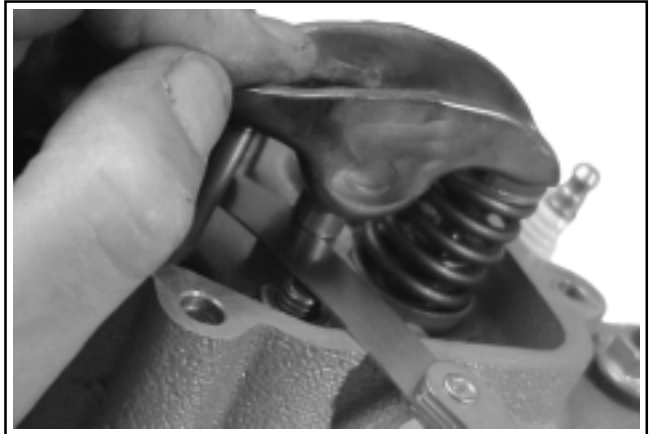
Figure 11-35. Determining Clearance with Feeler Gauge.
