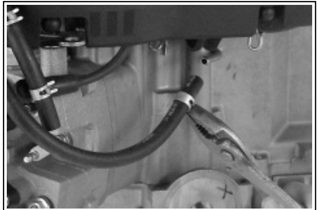
Figure 9-10. Disconnecting Pulse Line from Fitting.
