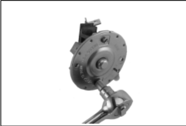
Figure 8-27. Removing Brush Holder.
