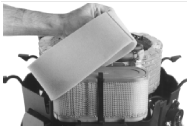
Figure 4-7. Removing Precleaner from Paper Element.
