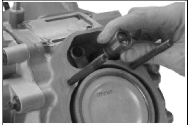
Figure 9-67. Removing Lifters from Lifter Bores.
