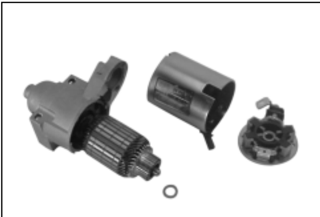
Figure 8-18. Starter Frame Removed.
