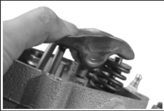
Figure 11-33. Depressing To Bottom Limit of Lifter Plunger Travel.
