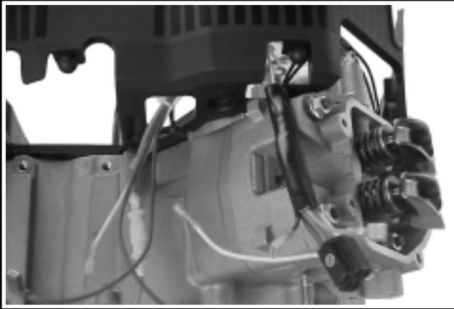
Figure 11-53. Wiring Harness out Through Openings in Lower Housing.
