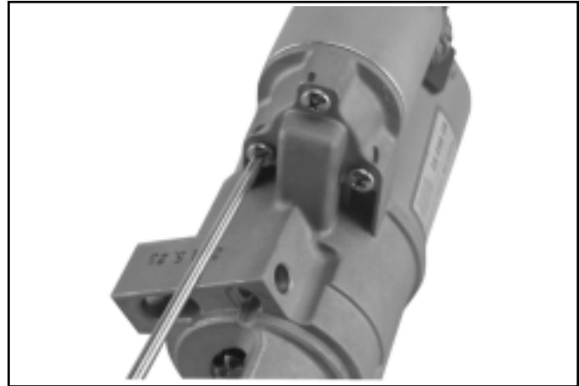
Figure 8-41. Installing Solenoid Screws.
