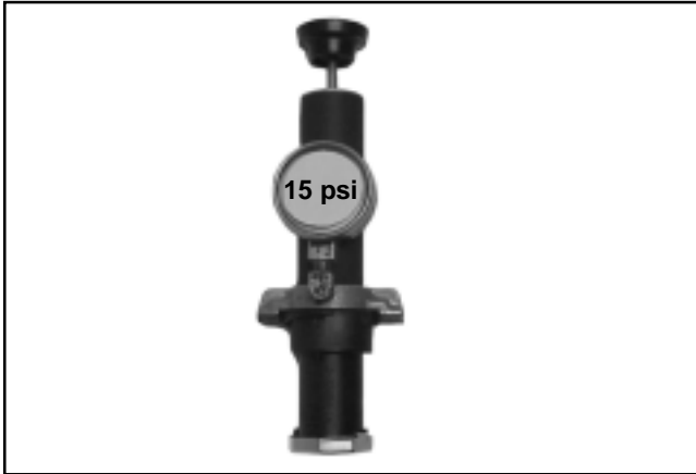
Figure 7-12. Adapter Installed onto the Tester.
