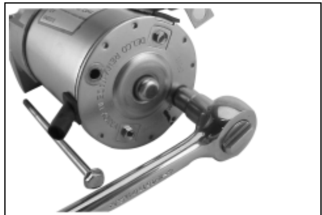
Figure 8-16. Removing Thru Bolts.
