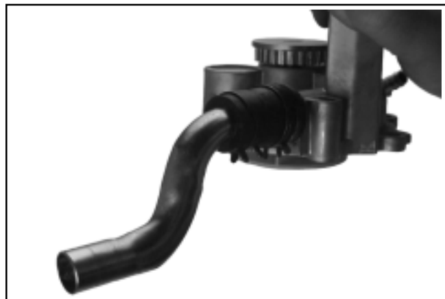
Figure 11-61. Tube and Second Clamp Installed.
