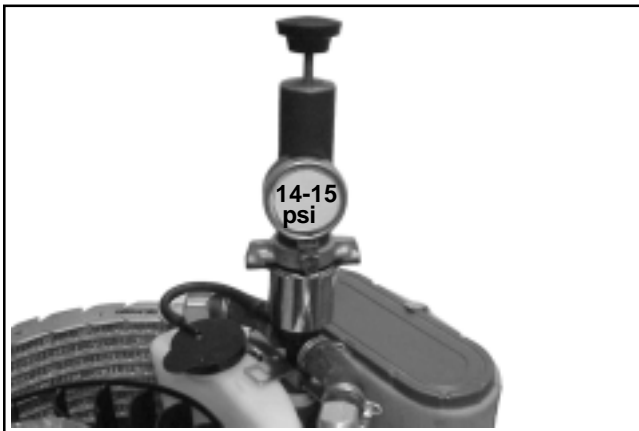
Figure 7-13. Adapter and Tester Installed.
