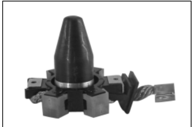
Figure 8-37. Brush Installation Tool with Extension.
