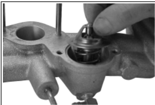
Figure 11-46. Installing Thermostat in Manifold.
