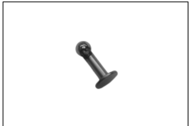
Figure 11-20. Tappet and Ball Bearing Welded Together.
