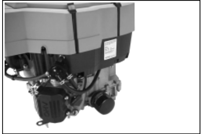
Figure 1-1. Engine Identification Decal Location.
