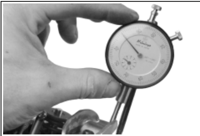
Figure 11-28. Align "0" with Needle.
