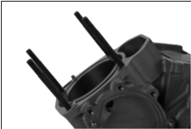
Figure 11-18. Side View of Crankcase and Studs for Height Dimension/Reference.
